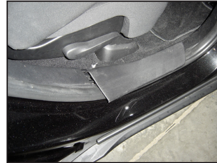
STEP 9 Remove the right rear door sill panel by carefully pulling up on the panel to release the clips.
