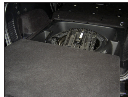
STEP 19 Reinstall the weather-stripping, door sill panel, plastic tub, and seat extension panel. Then, reinstall the padding, spare tire, storage pockets, and tool kit. Finally, reinstall the floor panel.
