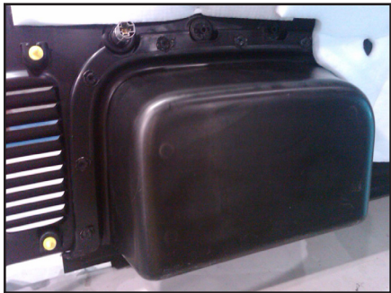
STEP 13 From the back of the side panel, the plastic welds that hold the pocket to the panel are visible.
