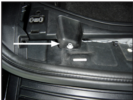
STEP 6 Remove the two hex nuts that hold the rear of the plastic tub in place.
