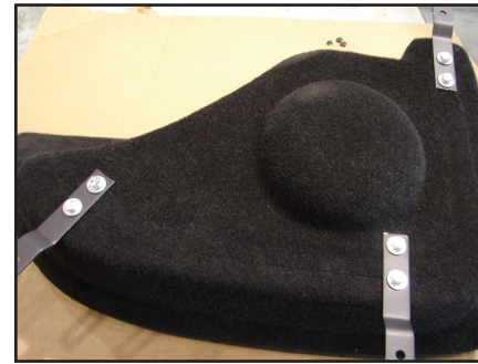
STEP 16 Using a pair of 1/4" Flat Washers, 1/4" Lock Washers, and 1/4-20 Hex Tap Bolts, attach each of the three brackets to the back of the Stealthbox as shown, and firmly tighten.
