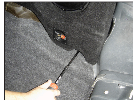
STEP 18 Thread a 6mm x 1.0 Flange Nut over the lower stud, and hand tighten.
