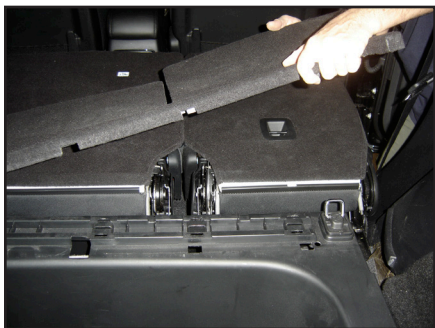
STEP 7 Remove the seat extension panel by carefully pulling up on the panel to release the clips.
